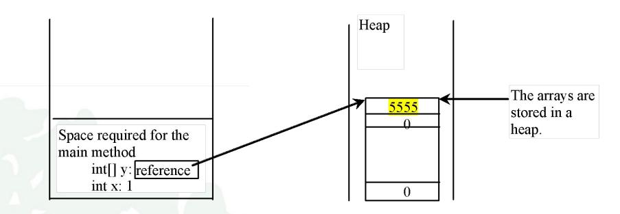
The JVM stores the array in an area of memory, called *heap*, which is used for dynamic memory allocation where blocks of memory are allocated and freed in an arbitrary order.
