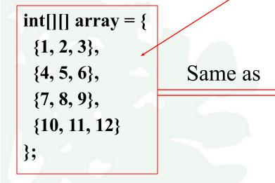
int[][] array = new int[4][3]; array[0][0] = 1; array[0][1] = 2; array[0][2] = 3; array[1][0] = 4; array[1][1] = 5; array[1][2] = 6; array[2][0] = 7; array[2][1] = 8; array[2][2] = 9; array[3][0] = 10; array[3][1] = 11; array[3][2] = 12;
