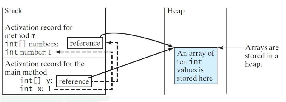
When invoking m(x, y), the values of x and y are passed to number and numbers. Since y contains the reference value to the array, numbers now contains the same reference value to the same array.
